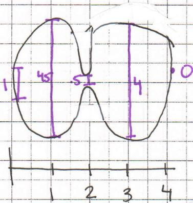
$$\begin{aligned} \text{Area} &= \frac{(1+4.5)}{2} \cdot 1 + \frac{(4.5+5)}{2} \cdot 1 \\ &\quad + \frac{(5+4)}{2} \cdot 1 + \frac{(4+0)}{2} \cdot 1 \\ &= \frac{1}{2} (1 + 2(4.5) + 2(5) + 2(4) + 0) \\ &= \frac{1}{2} (1 + 9 + 10 + 8) = \frac{1}{2} \cdot 19 = \frac{19}{2} \text{ in}^2 \end{aligned}$$
